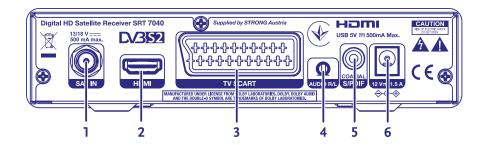
1. **SAT IN** To connect to the LNB of your satellite dish for reception of satellite broadcast
