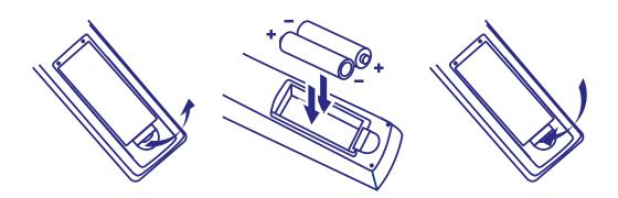
Remove the battery cover from the remote control and put 2x AAA size batteries inside the compartment. The diagram inside the battery compartment shows the correct way to install the batteries.
