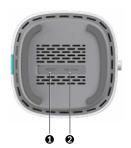
1. Reset button 2. Nano Sim card slot 3. USB 3.0 4. 2.5 Gigabit Ethernet Port (WAN/LAN) 5. Gigabit LAN Ethernet Port 6. Phone Port (RJ11) 7. On/Off button 8. Power Supply connector
